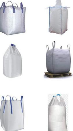
FIBC bags are manufactured by polypropylene woven fabrics that are stabilized against UV degradation. Each bulk bag can contain load capacities between 500kgs to 2000kgs with safety of 5:1 or 6:1 (5:1 is for Single use & 6:1 is for multiple use or for UN bags), depending on the bag design and size. Optional LDPE inner liner can be included to provide additional protection against moisture ingress.
